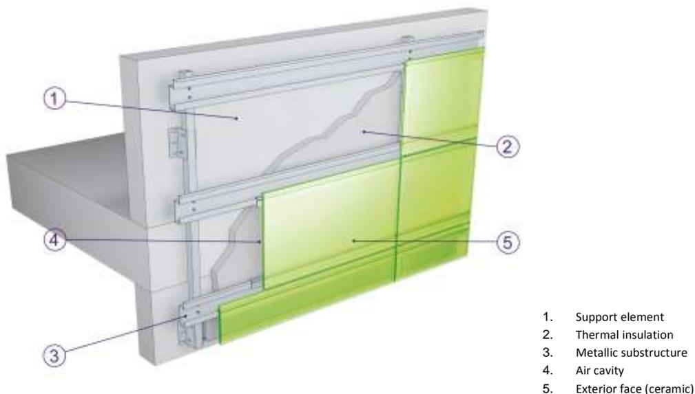
Figure 20. Parts of the façade
