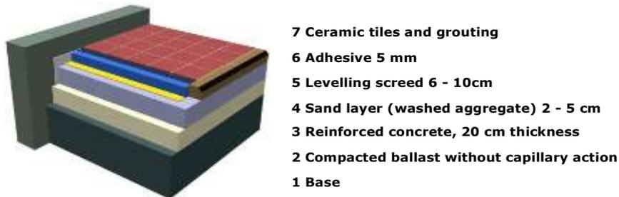
Figure 11. Paving system with thin layer over levelling base
