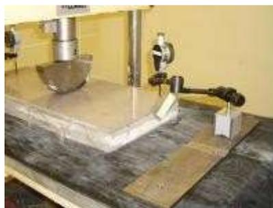
Figure 12. Concentrated load tests on poorly installed ceramic tile models
